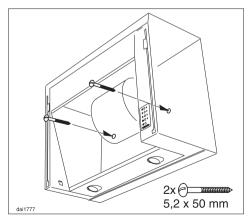
■ Fix the hood to the wall using the 5.2 x 50 mm screws provided.
